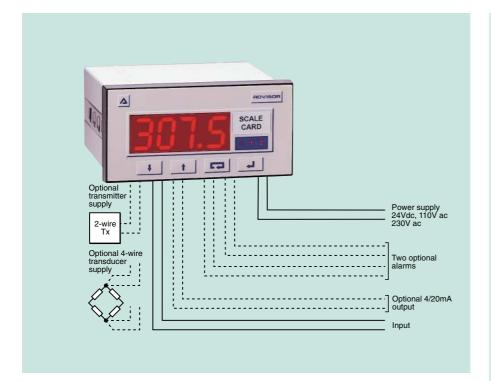
The Advisor A75 is a universal panel meter for displaying process variables in engineering units. In addition to the features offered by the fixed range A70, the A75 has twelve on-site selectable process voltage and current inputs. The meter is housed in a robust enclosure with high quality pushbuttons, display and terminals and will provide many years of reliable service.
